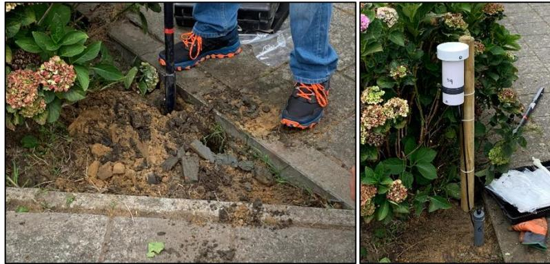
Figures 4 and 5: installation of the soil moisture, humidity and temperature sensors used in the SCOREwater project. On the picture we see digging of the hole where the soil moisture sensor is placed (left), and a measuring unit used by Measure Your City (right).
