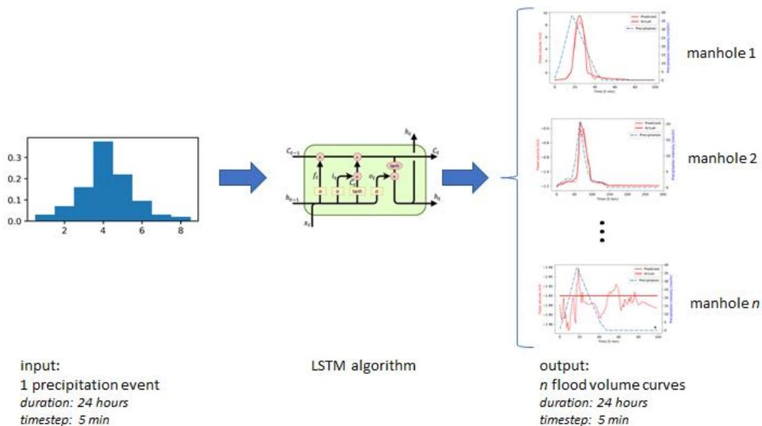
Figure 5: set up of the algorithm. A single precipitation event generates flood volume curves for each manhole in the network.
