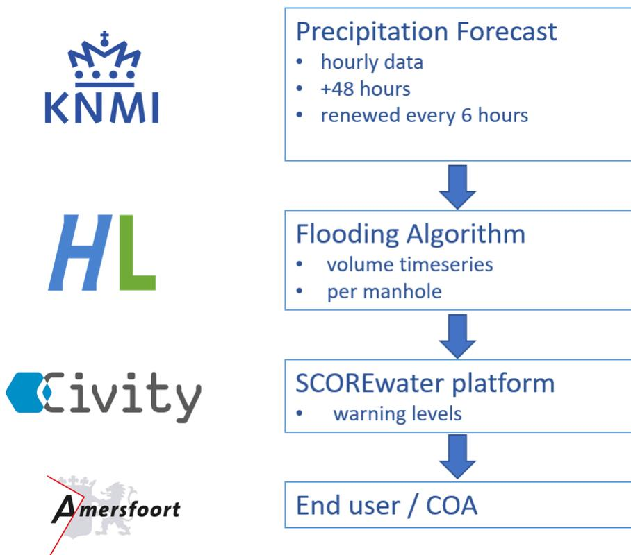
Figure 9: workflow of the flood early warning system, from precipitation forecast to a warning issued to an end user. This workflow is repeated every six hours.
