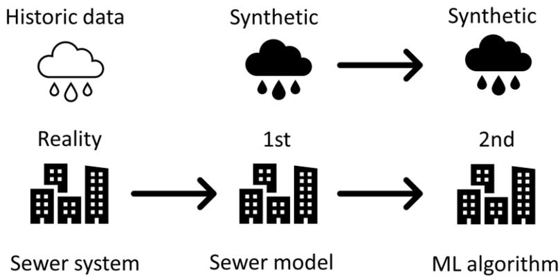
Figure 3: concept of the early warning system. A ML algorithm is trained on a data set created with a hydrodynamic model of the sewer system. The precipitation load is derived from extreme precipitation statistics for the Netherlands.
